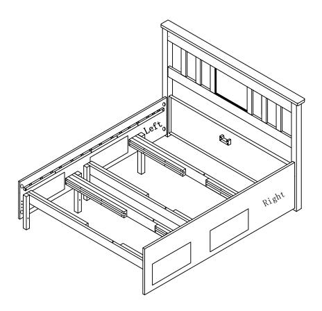
Step 5: Attach the Side Rails to the Footboard using the Half Moon Washer (B), Flat Washer (C), Hex Nut (D) and Spanner (E) please secure them into place and tighten, but do not fully tighten.
