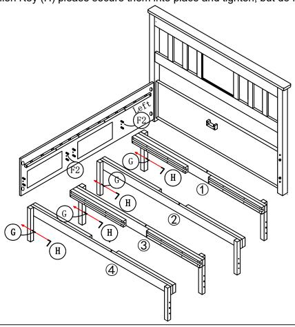
Step 4: Attach the Side Rail marked (Right) to the Headboard and repeat steps 1, 2 and 3.
