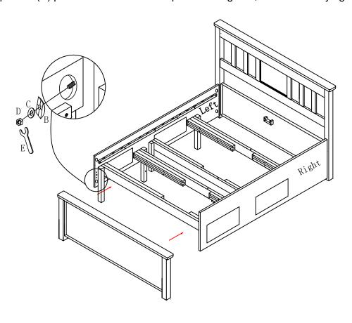
Step 6: Please Note Now the frame has been built, please ensure all fixing points are fully tightened using Spanner (E) and Allen Key (H).
