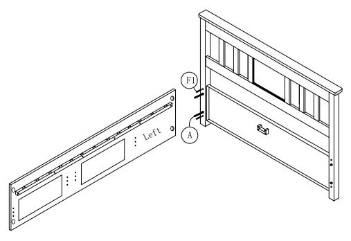
Step 2: Using the Half Moon Washer (B), Flat Washer (C), Hex Nut (D) and Spanner (E) please secure them into place and tighten, but do not fully tighten.
