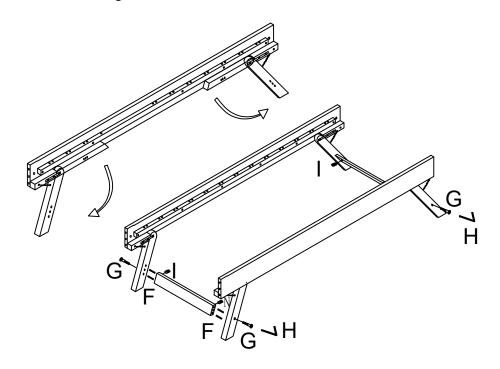
Step 2: Insert Wooden Dowel (F) and Barrel Nut (I) into the side rail and place the headboard into position securing with Bolt (G) and Allen Key (H) and then repeat on footboard.
