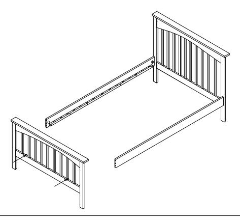
Step 4: Fit the Slat Cap (K) onto the Sprung Slat (L) and insert into the pre-drilled holes on the Side Rails, please note you may need to press firmly into place.
