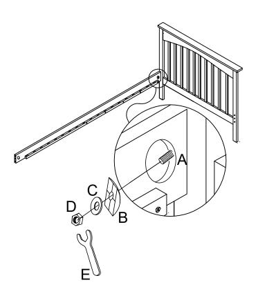
Step 3: Attach the Side Rails to the Footboard by repeating steps 1 and 2. Once the frame is secure, please tighten all 4 ends fully using the Spanner (E).
