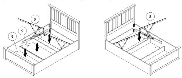
**Step 9**: Attach the bed base to the hydraulic frames using hardware part M. Fix the bolts starting from area 1 and finishing in area 3 – do not fully tighten the bolts yet.
