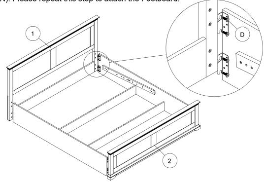
Step 3: Attach the Metal Corner Support (C) to the Footboard (2) and Side Rails using hardware (D & N).
