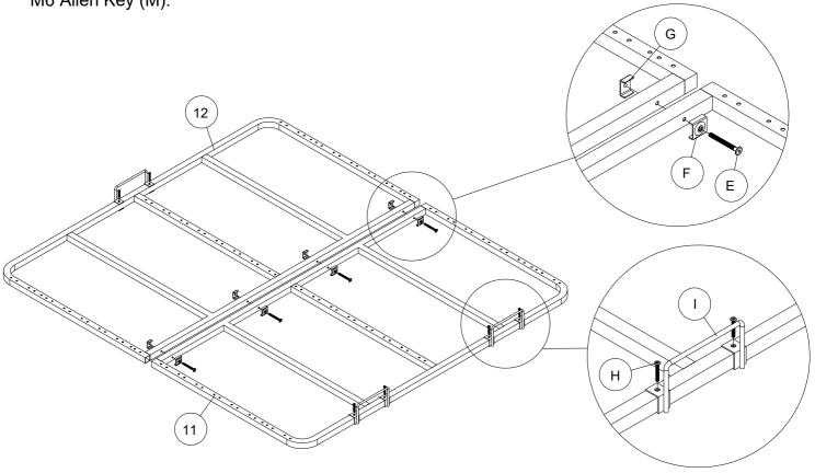
Step 6: Insert the Wooden Slats (13) into the Plastic Caps (K & L) and connect the slats to the Metal Base.
