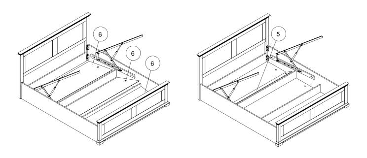
Step 8: Attach the assembled Metal Bed Base to the Hydraulic Base Supports (8 & 9) using hardware (J & N), but don't fully tighten the bolts. Start from headboard, then the middle and finally the footboard.
