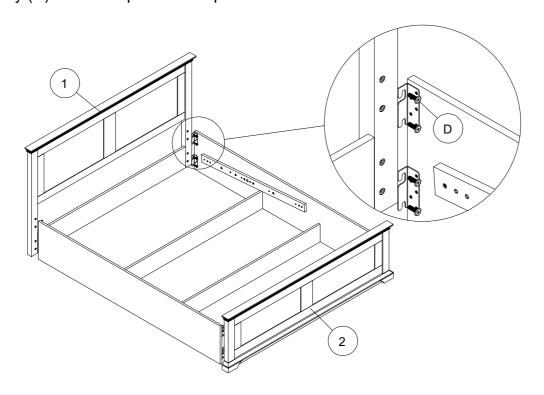
Place Metal Corner Support (C) to the Footboard (2) and Side Rails. Insert M8 x 16mm Bolt (D) and finger tighten. Ensure all corners are properly square (IE – At right angles) then fully tighten Bolt (D) using M8 Allen Key (N).
