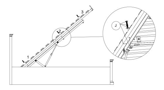
Step 9: Carefully lower the Metal Base using the Base Handle at the Footboard End. A moderate amount of force will be required, if necessary place your mattress on top of the Metal Base to assist with this.
